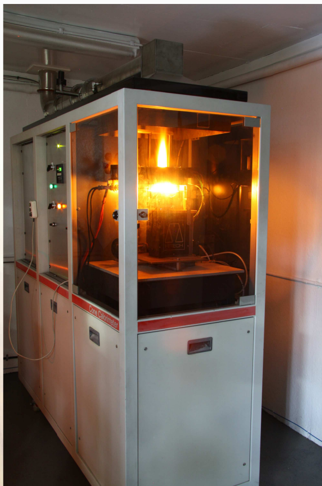
The new cone calorimetry test apparatus at Chiltern International Fire.
